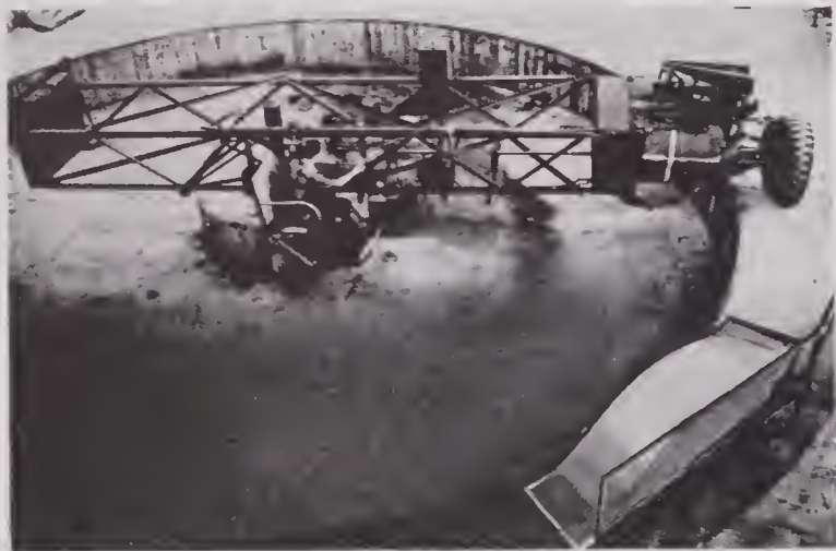
FIGURE 23. Merry-go-round setup for experimental wheel unit tests.
